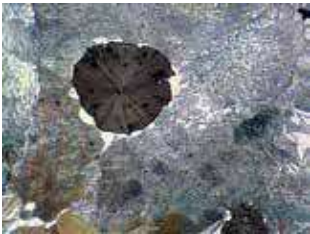
Pearlitic structure with nodular graphite, carbides and pearlite noduls
